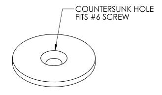
ZINC PLATED STEEL DISC FOR ATTACHING TO MAGNETS
